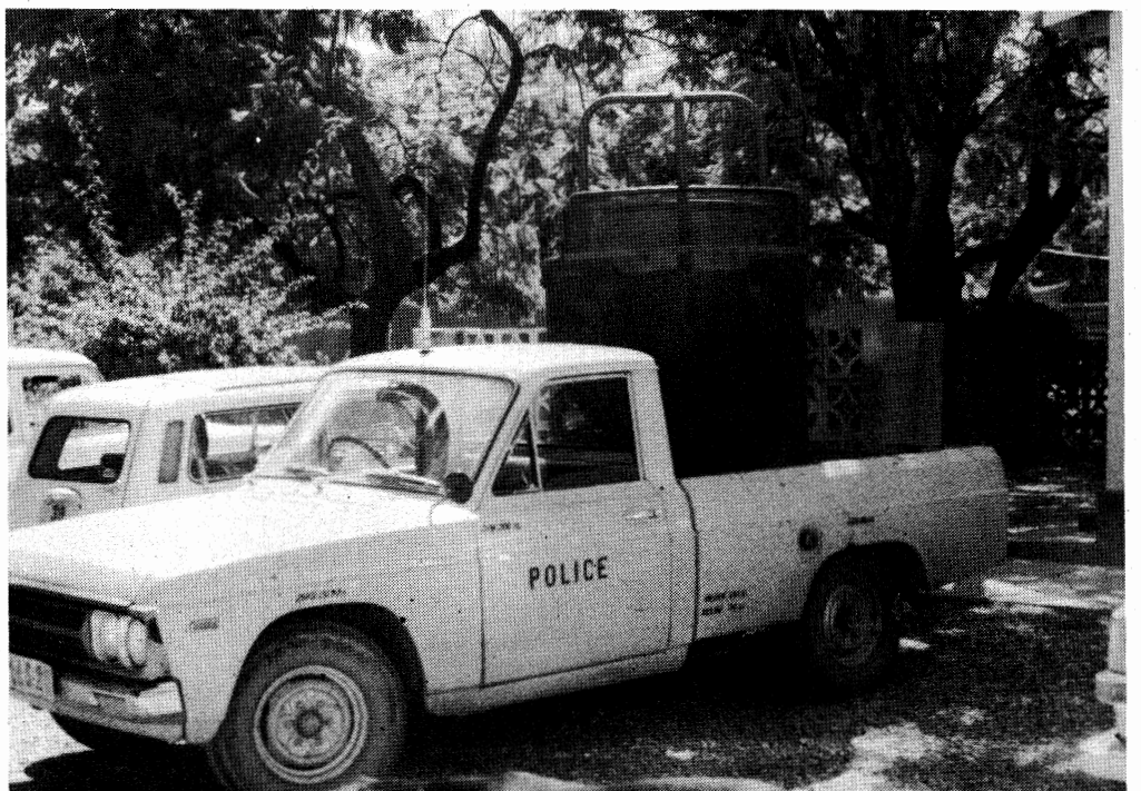
... A converted pick-up for convoy protection; a Browning machine-gun from a Spitfire is mounted on the tower.
