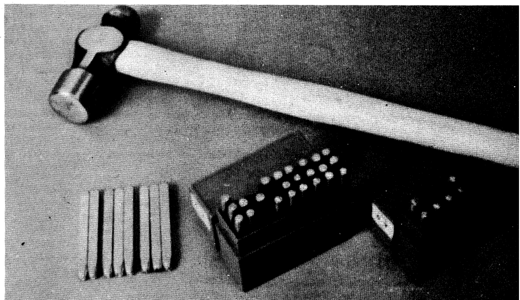
A hammer and die-stamps are all that is required to post-code the
